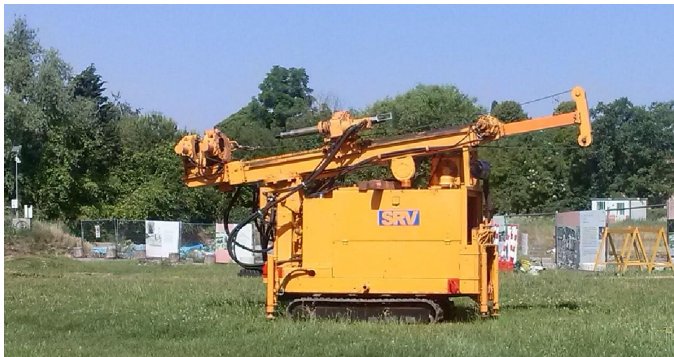
Sonda Atlas Copco A30 - SRV srl - 2014
